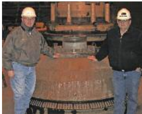
Bernie joined by Dale Kaskisko of Frog Switch inspect a Frog manganese bowl and mantle at a local mine.
